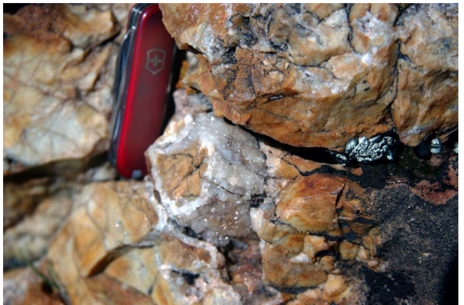
Fig. 3.11. Close-up of building blocks of the Watch Tower showing glistening quartz crystals in cavities. With a magnifier, the frosty coating resolves into tiny, perfectly formed quartz crystals that grew into open spaces of the chert/agate rubble during its long burial history. All spaces between the rubble were partially or totally filled with innumerable quartz crystals. The pocketknife is about 2" long.
