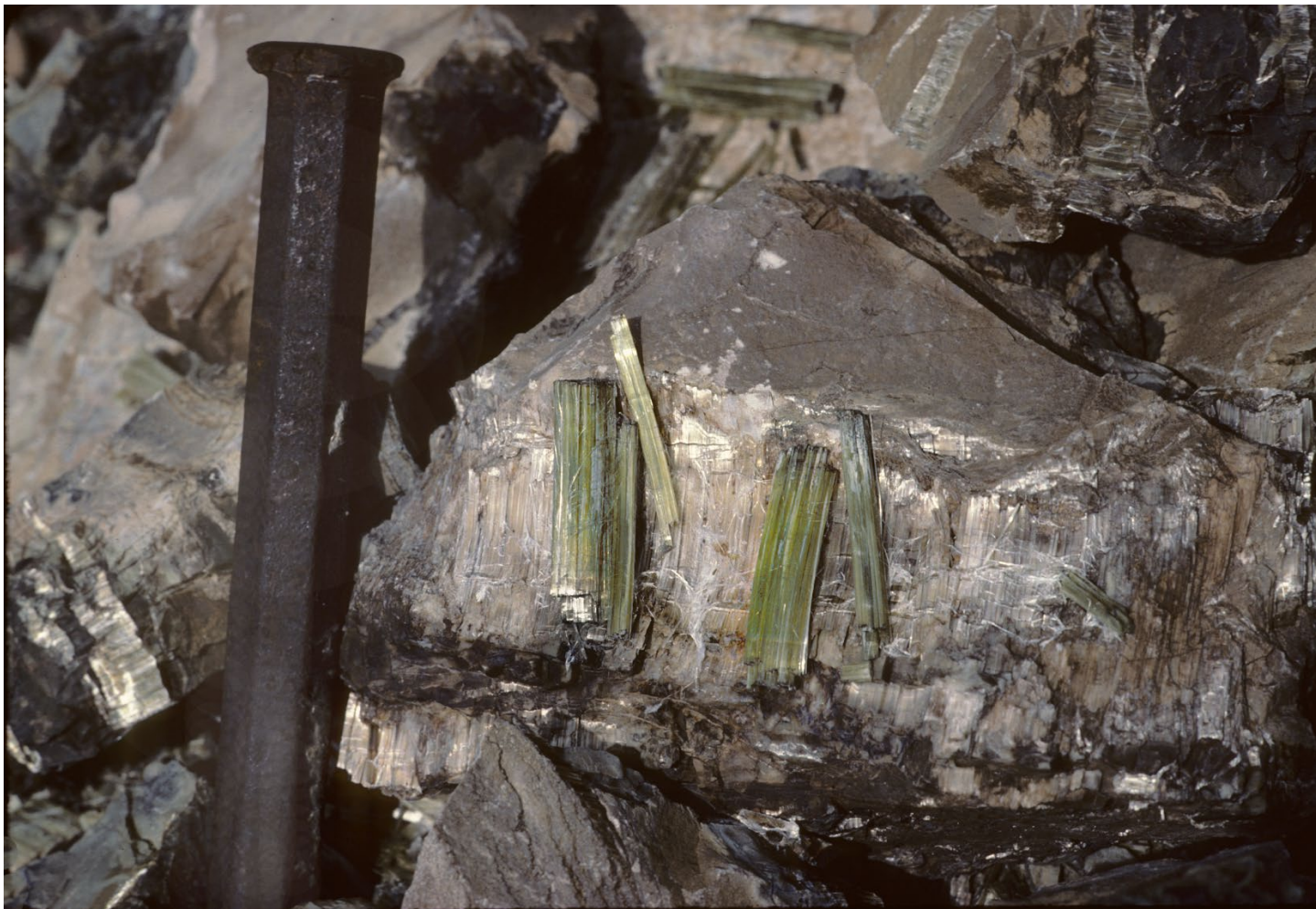
Fig 16.10. Beautiful fibrous chrysotile asbestos at the digging near river level. The spike from the mining activity in 1910 is \frac{3}{4} " wide.
